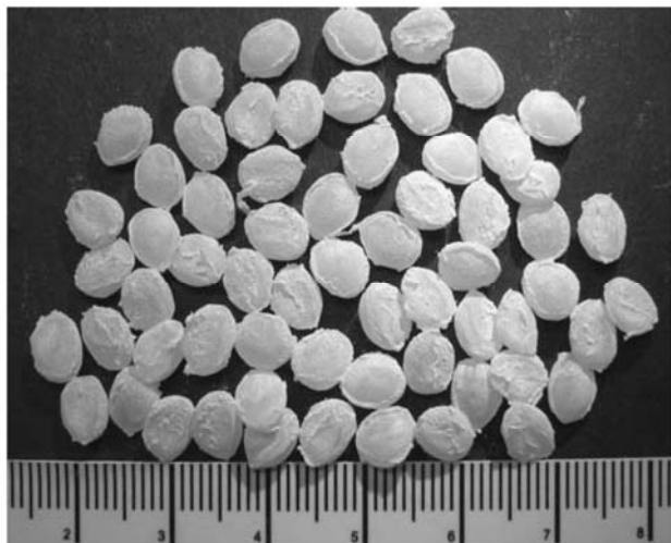
Fig. 1. Fluororubber Elaftor 3000. Fluororubbers Elaftor of series 2000 (Elaftor 2031, 2041, 2051, 2061, 2071, 2081) are copolymers of vinylidene fluoride and hexafluoropropylene containing 66 wt% of fluorine, density 1.83 \text{ g cm}^{-3} , glass transition temperature -17^\circ\text{C} , curing with bisphenol or amine.
